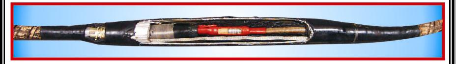
PILC Heat Shrink Joint rely on Irradiated Polyolefin Oil barrier & Insulating tubing which prevent impregnation / Ozoing of oil & grease from the paper insulation of cores, built up better Insulation over the cores & Metallic cannister with outer jacket tubing protect the joints from outside.
