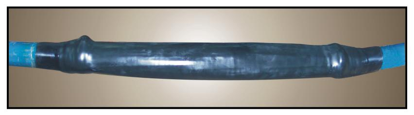
'Cabseal' Heat Shrinkable Type Joints & termination rely on the insulating & sealing properties & on Inline connector region which is being enhanced by a unique mastic tape and irradiated polyolefin tubing being easily & effectively applied by any common person. An elastomeric core separator enhance the insulation and sealing system of the joints.
