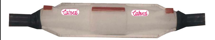
Straight joint designed for direct burial under the ground design consist stress control pad. Highly insulating self amalgamating EPR tapes & Polyurethane based compound for mechanical protection & sealing of cable against ingress of moisture & water.
