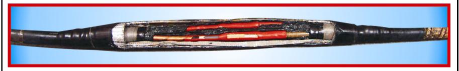
Transition Heat shrink St. Th. Joint is a unique combination for joining PILC Cable to XLPE Cable. The Joints consist Irradiated Polyolefin Oil barrier tubing on PILC side to avoid the impregnation /oozing of oil and grease from the paper insulation of cores. Yellow mastic & Irradiated Polyolefin red insulating tubing are controlling the stresses developed on XLPE side & provides better insulation.
